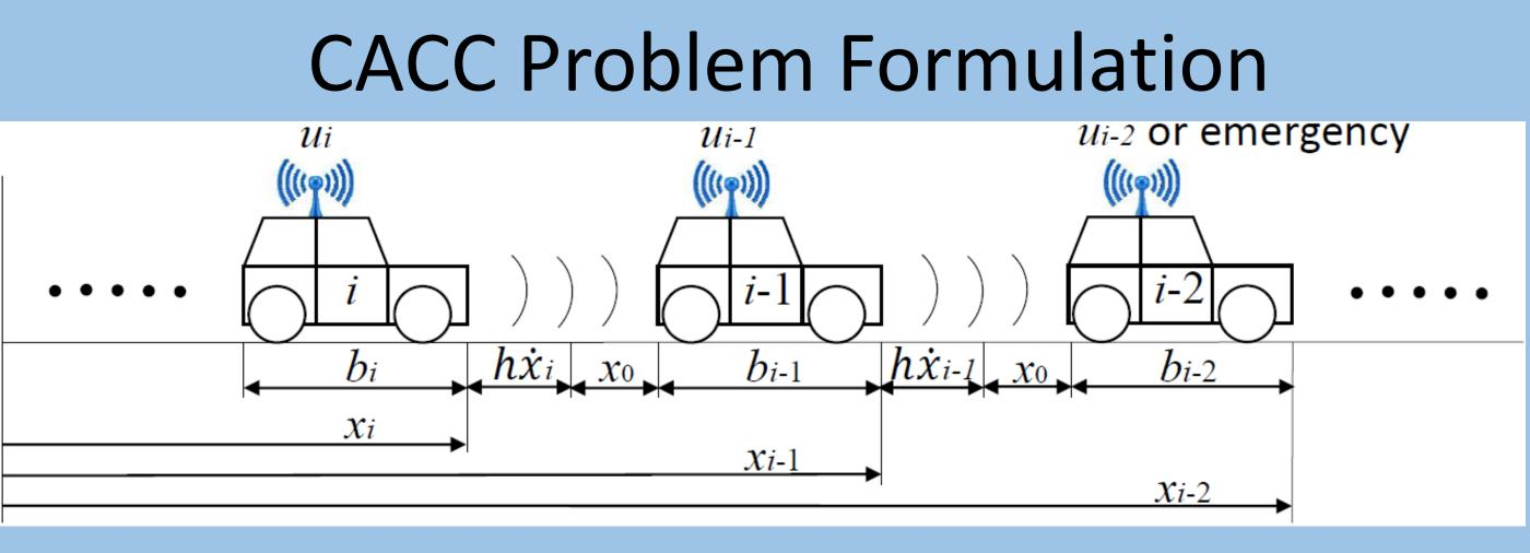
The desired intervehicular distance is  $x_0 + h\dot{x}_i$  where  $x_0$  is the standstill safety distance and h is the constant time gap. > The control system minimizes the error between the actual and desired distances.
