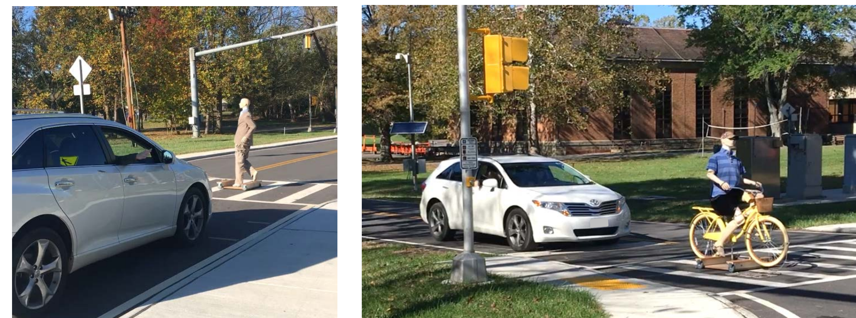
Figure 2a and 2b. Testing the validation system with simulated walking pedestrian (left) and bicyclist (right). Source: FHWA
