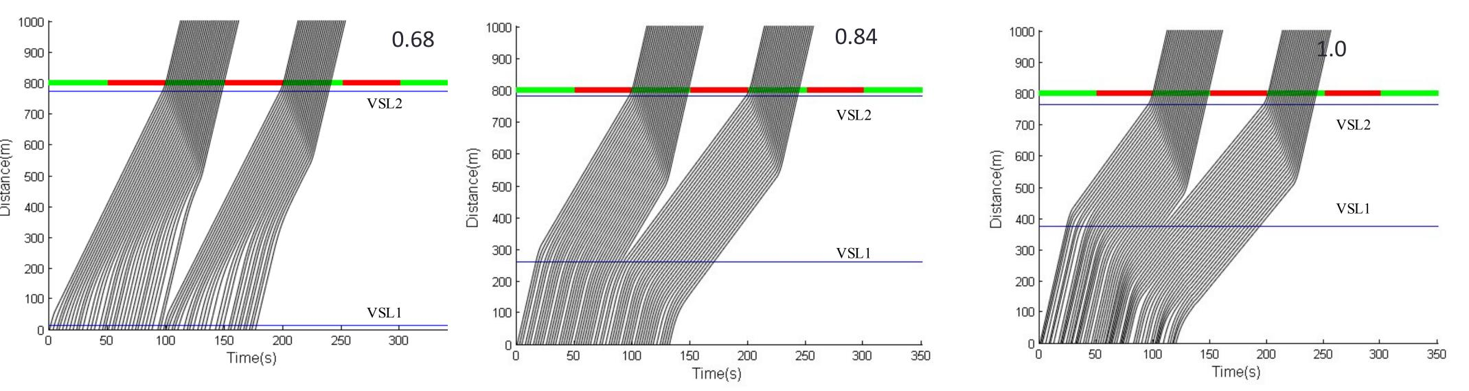
ASL may cause excessive queue spillback under dense traffic conditions. LTC can circumvent this disadvantage by optimally setting the speed slow down point according to traffic volume.
